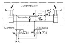
Port T can be connected with the unclamping line, when that line is without pressure during the clamping process.
