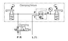
When using a pressure reducing valve with reservoir connection, always a 2nd line is required to connect port T with port L or R at the power unit.
