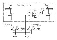
The easiest way is to install a third line from port T of the pressure reducing valve to port L or R of the power unit.
