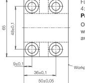
Fixing screws 4x M8x25 12.9
