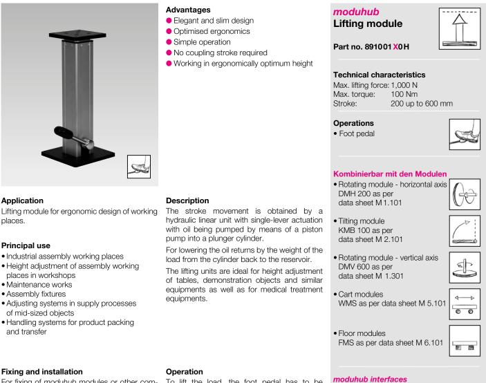
For fixing of modulub modules or other components of the user at the top plate the lifting module has an interface 140 x 140.
