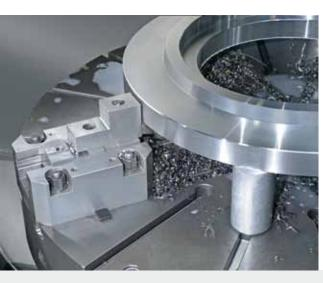
For holding workpieces in milling and turning centres, HILMA box jaws are the first choice. This new development combines a number of striking advantages compared with the normal level of technology available in the market.
