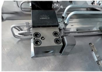
Wedge clamp with hydraulic ports  ${\bf A}+{\bf B}$  at the right and an additional cooling circuit  ${\bf C}+{\bf D}$  at the opposite, left side
