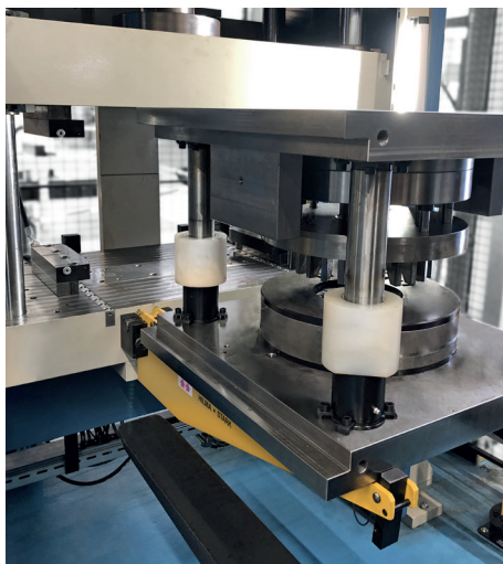
Clamping bars installed in press bed and ram. Easy loading of dies by die changing consoles and hydraulic ball bars installed in the T-slots of the press bed.
