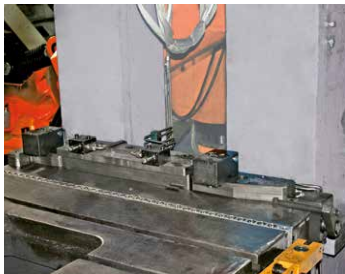
Clamping block separately mounted on bars, ball bars in the press bed, carrying consoles in front. Block cylinders and swing clamps for positioning
