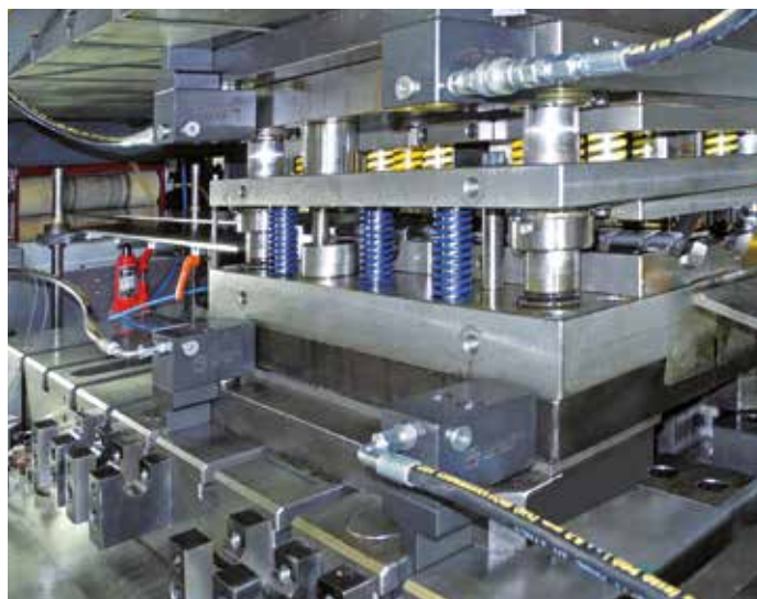
Sliding clamp with T-slot adapter in press bed and ram, roller bars and carrying consoles for tool insertion
