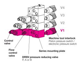
**Valve block** (max. 4 control circuits V1–V4) The equipment of the control circuits is based on the functional requirements of the application. The maximum pressures as well as the design-related differences in poppet and spool valves are to be considered.
