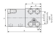
Installation of drill bushings to absorb side loads The occurring side loads must be absorbed by drill bushings to be inserted into the fixture plate.
