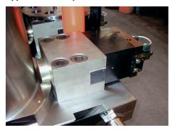
Wedge clamps on a forging press
