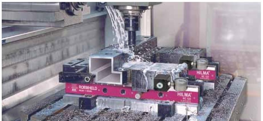
Clamping of sensitive workpieces without deformation (housing parts)
